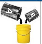
Add A component and B component at the specified 2A:1B ratio in a clean 5-gallon bucket.
