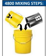
**Pour pre-mixed A-Component** and B-Component into a clean 5-gallon bucket (If mixing bulk kit be sure to follow specified 2A:1B ratio)
