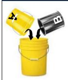
Pour pre-mixed A-Component and B-Component into a clean 5-gallon bucket (If mixing bulk kit be sure to follow specified 2A:1B ratio)
